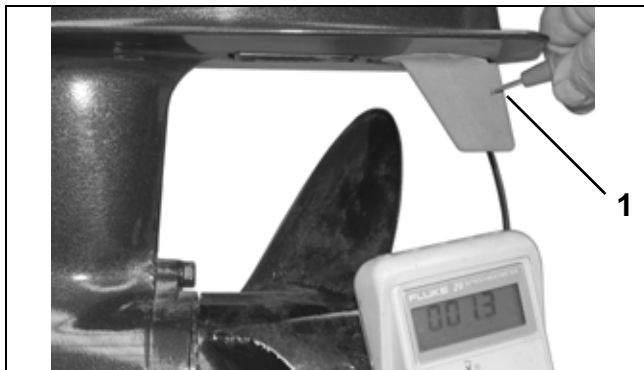
1. Meter lead to anode
